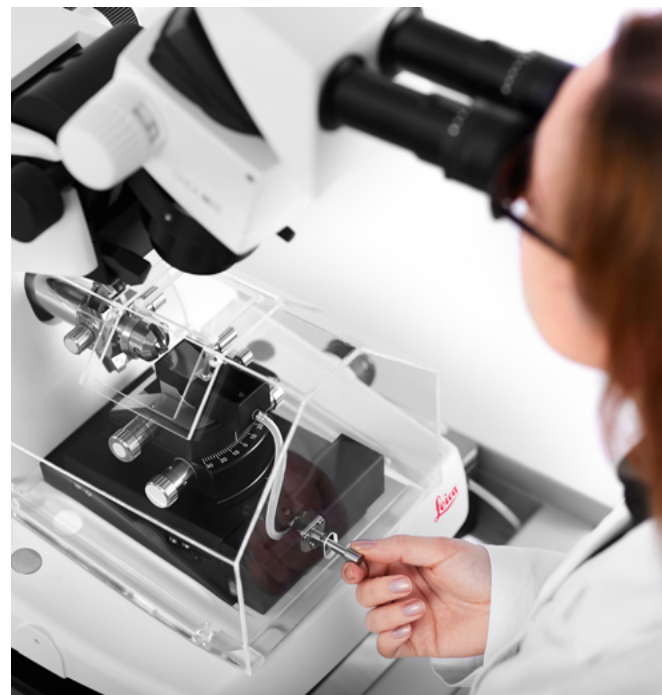
Avoid ribbon wrinkling by simply adjusting the ARTOS 3D front valve to control the water flow rate. More consistent section thickness is also attained with the ARTOS 3D draft shield and active damping system.
