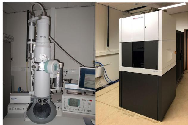
The TalosF200i is a versatile transmission EM with sub-nanometer resolution. MAPS software is capable of recording and stitching multiple images. It is also equipped with detectors for elemental detection, aka '[ColorEM](#)', as well as automated tomography: 3D imaging at the nanoscale. The CM100 is no more...
